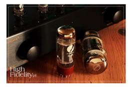
L One may use various tubes in the EVO 200 – photo shows Tung-Sol KT120 beam tetrodes
